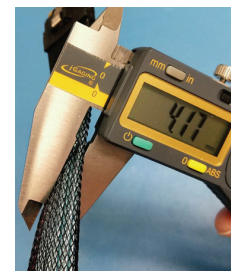
Standard individual twinax SlimSAS 8i
